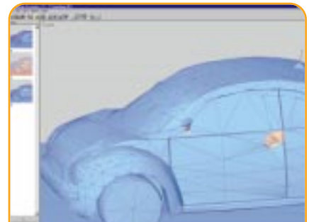
FIGURE 3. Decimator mercifully allows the artist to reduce triangle count in a particular area, as seen in the rear-view mirror here.
