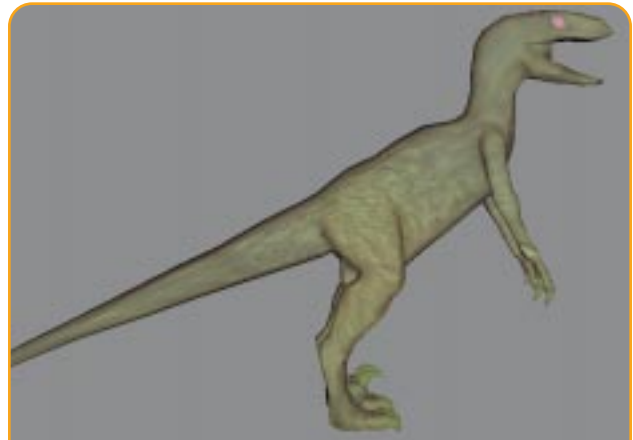
FIGURE 1. This shows NetImmerse's continuous LOD demo. As you move the dinosaur into the distance, its polygon count decreases. Popping is scarcely visible.
